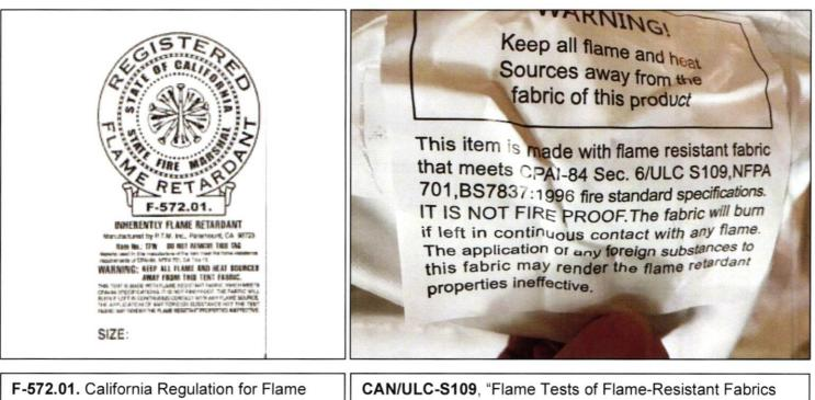
**F-572.01.** California Regulation for Flame Spread Rating: tent label accepted by Cavan Monaghan Fire Department **CAN/ULC-S109**, "Flame Tests of Flame-Resistant Fabrics and Films", <u>or</u> **NFPA 701**, "Fire Tests for Flame Propagation of Textiles and Films": tent label accepted by Cavan Monaghan Fire Department
